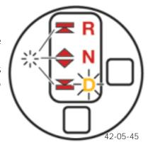
This display is illuminated when the transmission is in the *mechanical emergency operation* and in the P position. All of the arrows will flash at a frequency 1.5 Hz. The shift pattern locator illumination for R, N, D will remain on and the P position is indicated.
